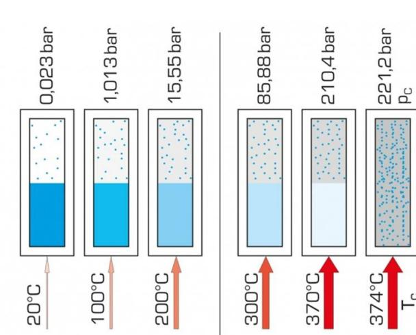
Heating up water in a closed tank: the pressure and temperature increase proportionally up to the critical point, at which fluid and vapour are no longer distinguishable from each other; critical point at T<sub>c</sub>=374°C, p<sub>c</sub>=221bar, dotted line: temperature limit of the experimental unit
